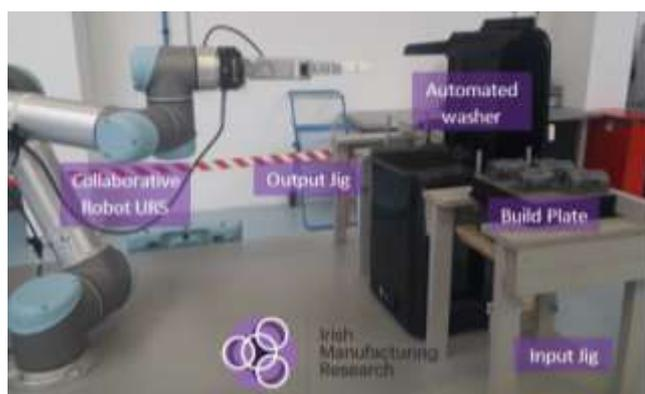
Figure 1 - Cell Setup
